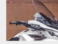
**ADJUSTABLE ELECTRIC WINDSHIELD:** Wide range of wind protection and adjustable with the push of a button.
